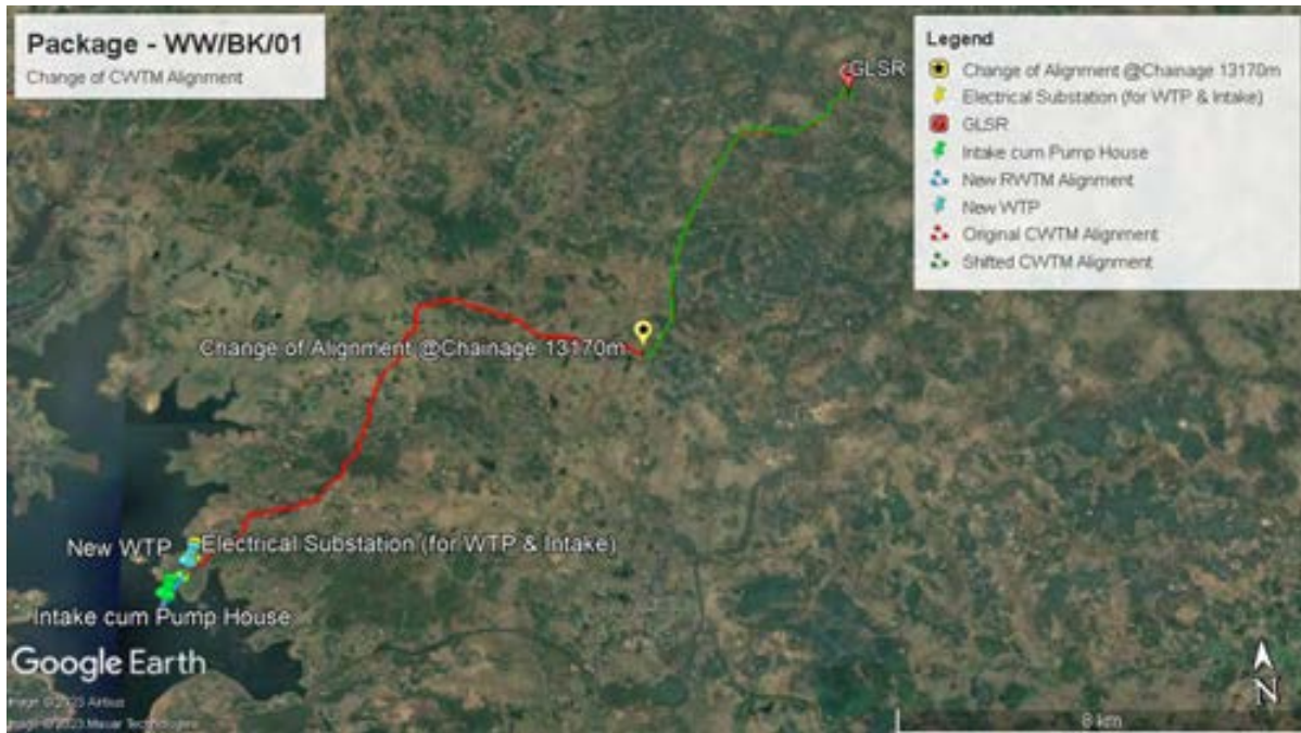
GLSR – Ground Level Storage Reservoir, WTP – Water Treatment Plant, CWTM – Clear Water Transmission Main, RWTM – Raw Water Transmission Main. Source: DSISC, Bankura
